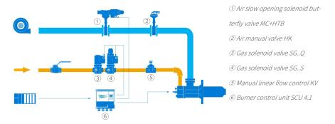
In on/off pulse control mode, SFID 90N~320N can be ignited directly at maximum capacity.
