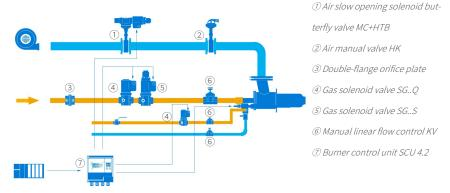
■ In on/off pulse control mode, a pilot burner is recommended for SFID 450N~630N, which is used for ignition and flame detection.
